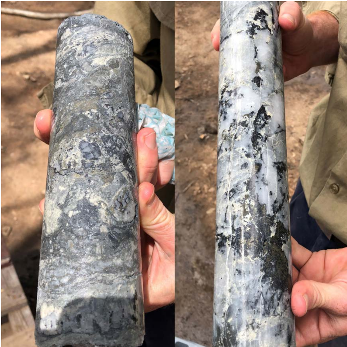
Figure 4. Left Image: sphalerite, galena and pyrite in matrix of breccia (~695m). Right image – black sphalerite in quartz vein (~699m depth)
