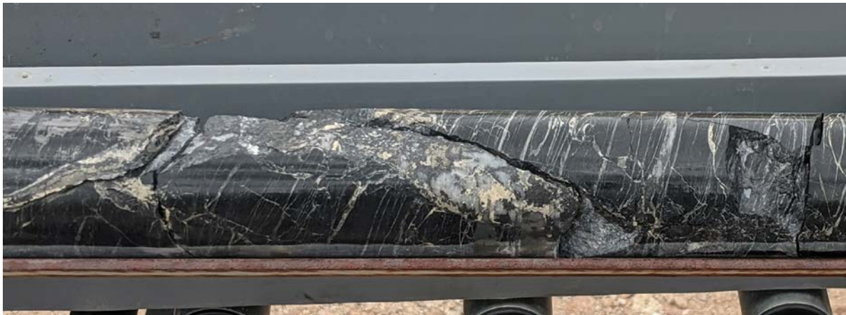
Figure 1. Semi massive sphalerite-pyrite veins and stringers overprinting quartz within silicified shale (~640m).
