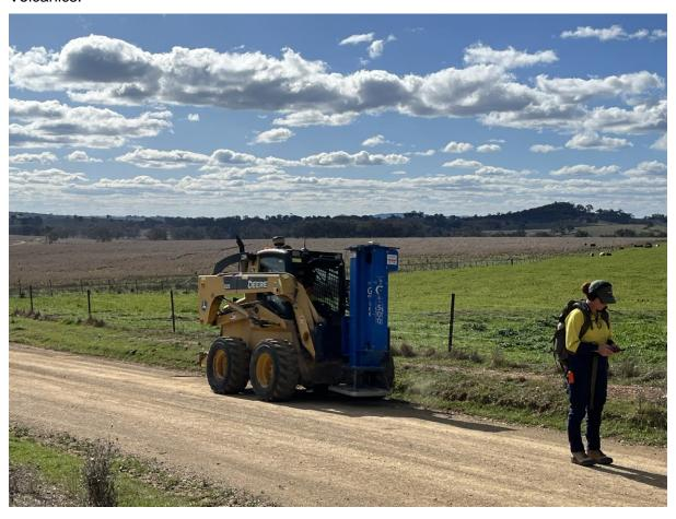
Figure 2: Seismic survey at the Barabolar Project with the pyrophyllite quarry in the background.
