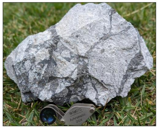
Figure 3: Material from bulk sample site with grey fracture/breccia fill minerals of silver sulphides such as acanthite (Ag<sub>2</sub>S), galena (PbS), sphalerite (ZnS).
